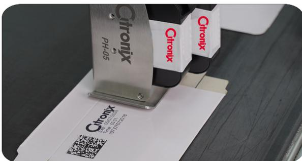
Using proven and reliable HP Thermal Inkjet 2.5 Technology and automatic parameter settings using smart ink technology we ensure you always have a reliable uptime.
